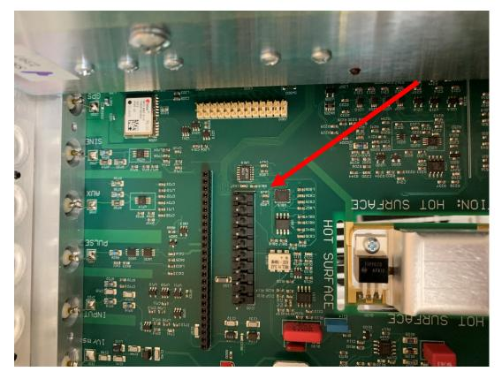
If the clock option chassis and the FS740 chassis do not line up flush (parallel), then you have installed the clock wrong (missed a pin), and you will need to remove the clock and then install it again.
